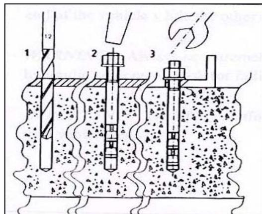
Fig 3.4 The lifting platform must be anchored to the floor
