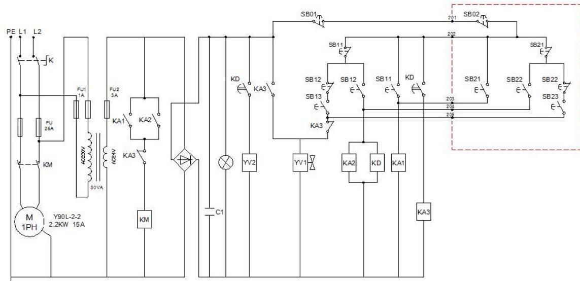
SB01 ,SB02: Emergency Stop Switch      SB11 ,SB21: Raising      SB12 ,SB22: Unlocking/Lower
